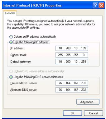
To change to DHCP first click in the 'radio button' next to 'Obtain an IP address automatically'
